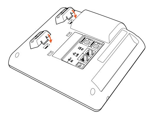
C. After install the wall-hung stand bracket, press one-side joints of stand bracket into the slot, please refer the picture as below:
