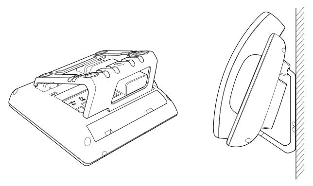
G. Disassemble the stand bracket:
