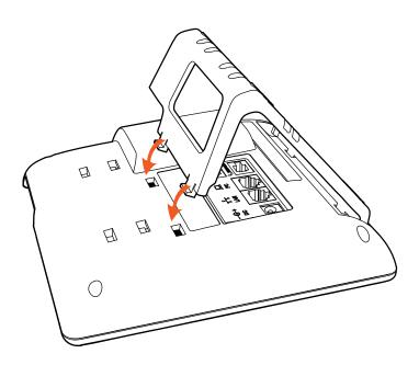
C. It is the right picture after fixing the feet below:
